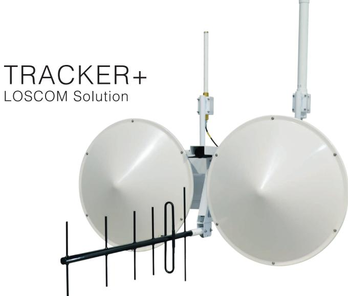
S-PLANE's TRACKER+ is the latest evolution of S-PLANE's very successful TRACKER 100 solution. It is a stand-alone GNSS-based antenna tracker with integrated primary and secondary software defined mesh network radios and a combination of directional and omni-directional antennas. Clients can select their configuration from various radio and antenna options to customise the solution to their applications. The TRACKER+ is able to dissipate the heat generated by specialised high-power radio systems.
